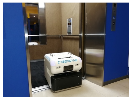
CL02 riding on elevators automatically
