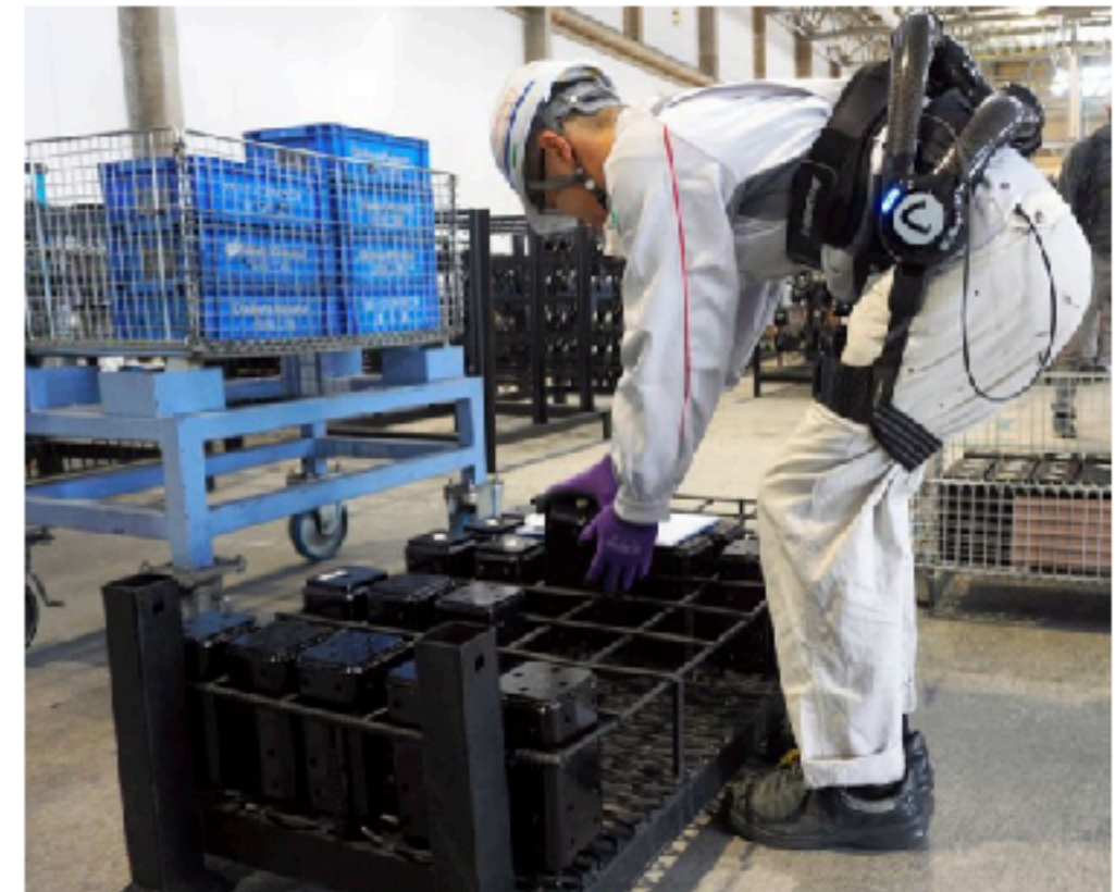
A worker wears a powered exoskeleton "robot suit" during physical work at the Daiwa House Industry Co. Nara plant on April 10. (Yoshikatsu Nakajima)
